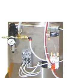
Complete with Pneumatically actuated discharge valve that ensure complete sealing and a solid state demand proximity sensor for auto fill.
